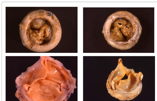
Figure 1: (Upper panel) Porcine bioprostheses explanted because of stenosis due to cusp stiffening ( left ) and regurgitation due to cusp tears caused by calcific infiltration ( right ). (Lower panel) Pericardial bioprostheses replaced because of regurgitation due to fatigue-induced commissural tears.
